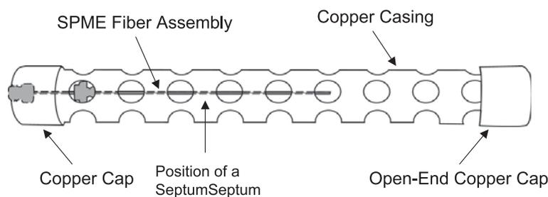
**Figure 2. Schematic of the SPME-based sampling device.**
