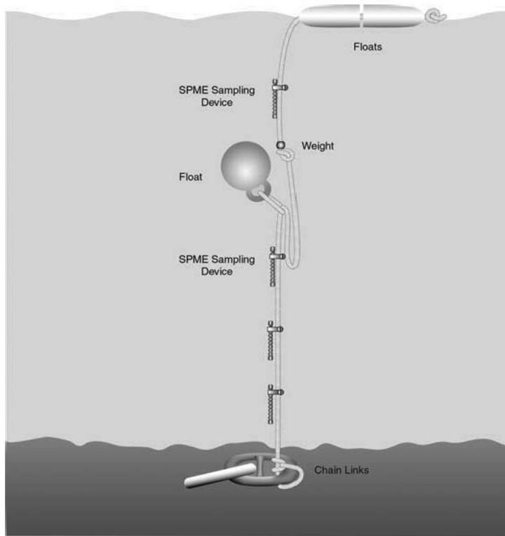
**Figure 3. Schematic showing the field deployment of SPME samplers at various depths in the water column.**
