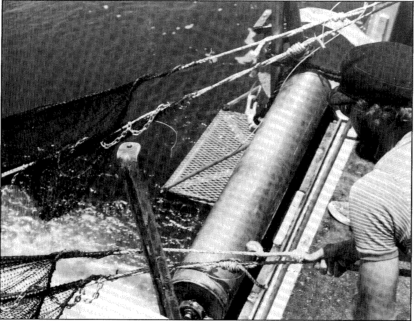
Retrieving the otter trawl
