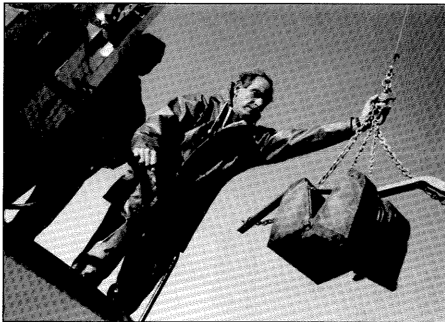
Jack Anderson deploys a Van Veen Grab to collect a sediment sample.
