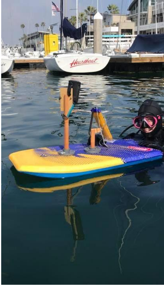
Figure 1. Surface personnel following bubble trails of underwater personnel with GPS tracking unit mounted to a floating board to record the perimeter of the eelgrass bed.
