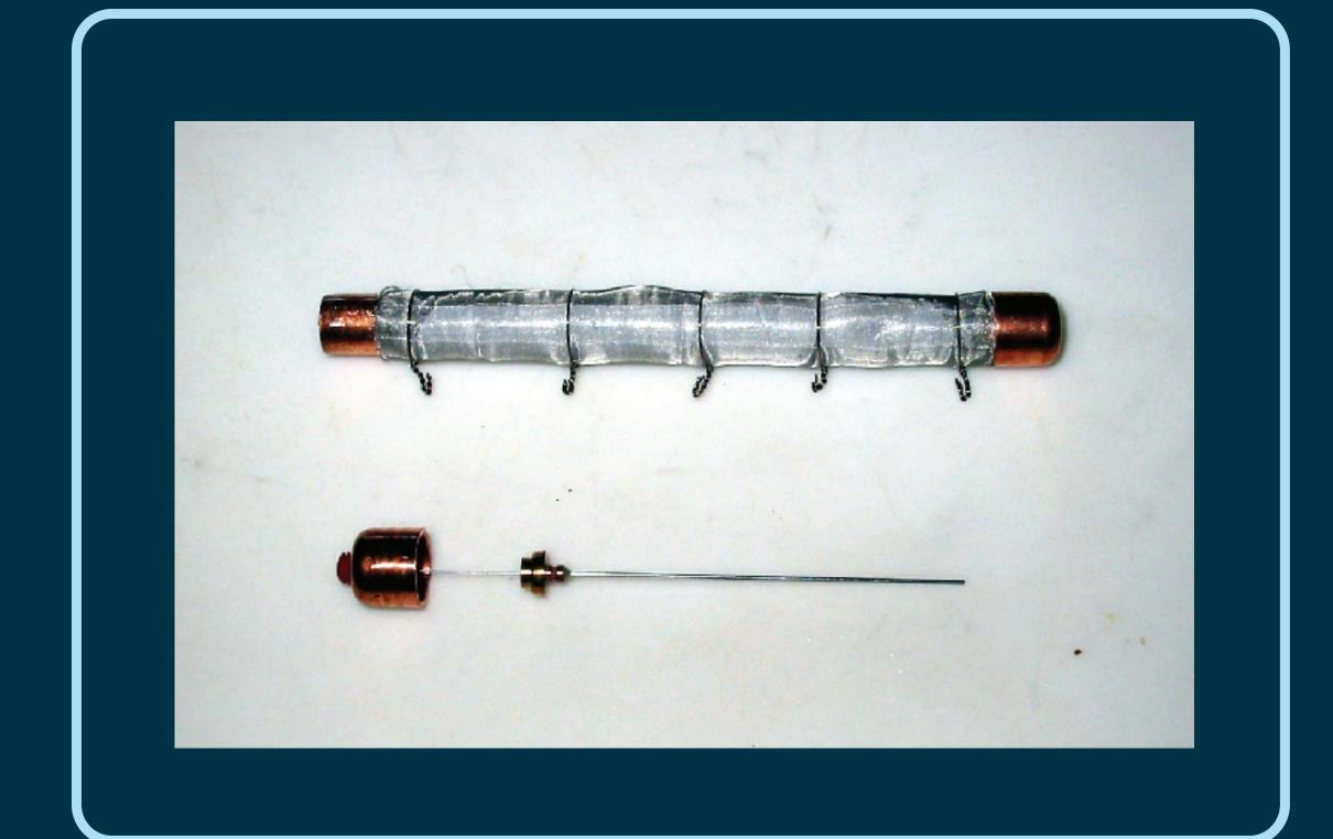
Fig. 1. SCCWRP's porewater sampler for HOCs (unassembled). (top) Copper housing with glass fiber filter and stainless steel mesh particle barrier; (bottom) SPME fiber (100 um PDMS) assembly attached to housing end cap.
