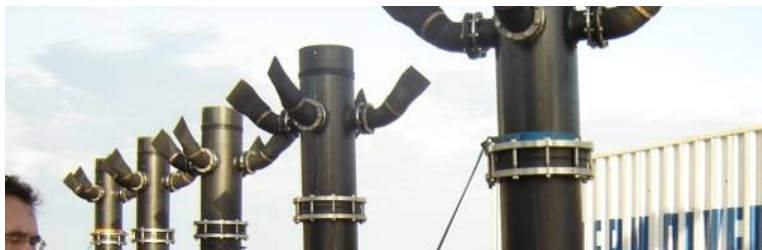
Figure 6-3. A rosette multiport brine diffuser.
