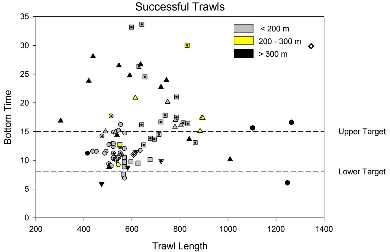
**Figure III-3. Tow distance versus net on-bottom time (pressure-temperature sensor) for successful trawls during the Bight'08 regional survey. Colors represent depth. Symbols represent vessels and field crews. The upper and lower bounds were the quality assurance goals prior to the survey. Five-minute tows omitted from graph.**
