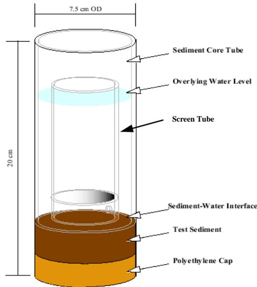
**Figure II-2. Schematic diagram of sediment-water interface exposure system (Anderson *et al.* 1996).**
