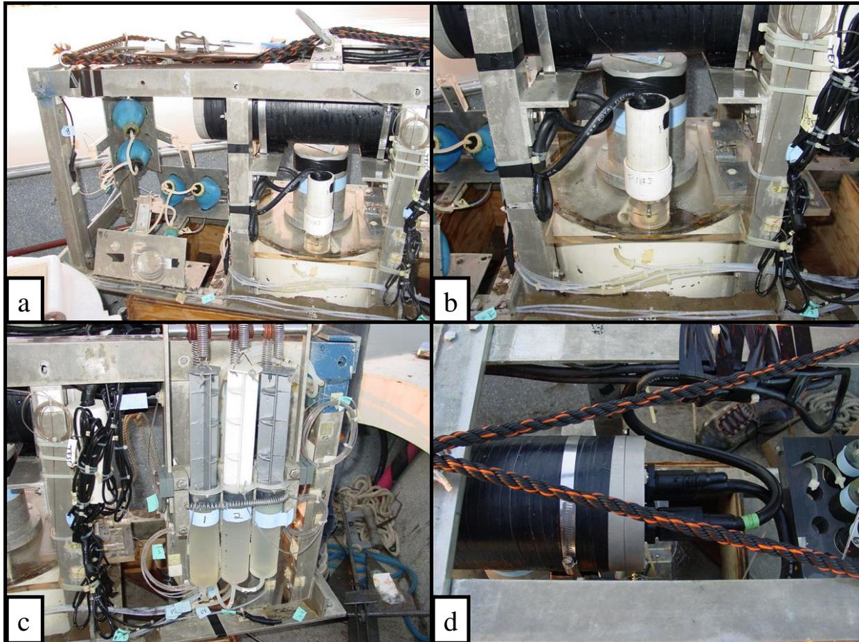
**Figure 3-1.** Photos of the benthic chamber apparatus mounted on an aluminum frame (a). The chamber body is constructed of polycarbonate with a clear acrylic lid; O<sub>2</sub> and temperature are measured directly within the chamber (b). Samples are drawn from chamber via spring-loaded syringes and flexible bulbs that are coupled to springed hinges (c). A data logger, contained within a pressure case (d), records all ambient data as well as all chamber mechanical operations.
