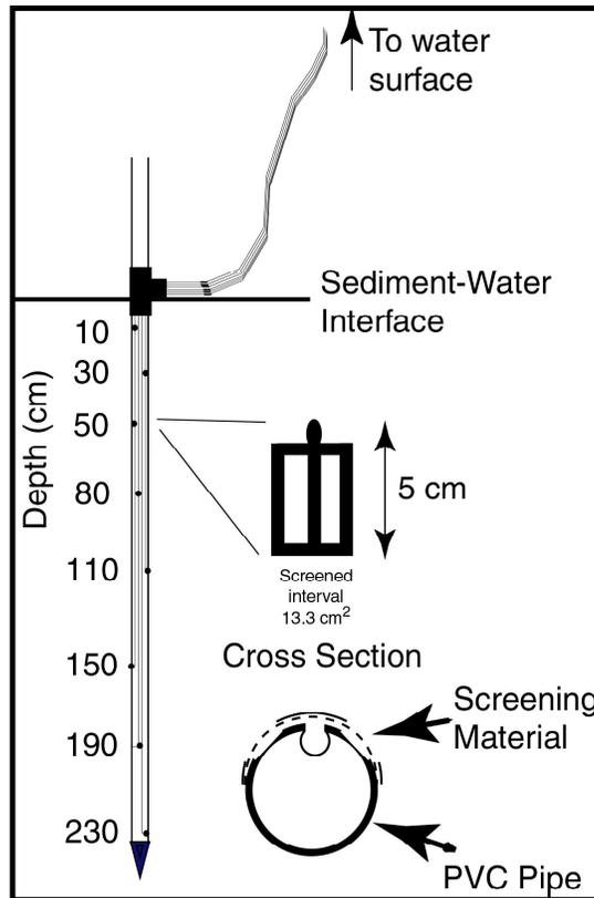
**Figure 3-2. Multi-level piezometers each contained eight sampling ports screened to 200 cm and connected to the surface via individual sampling tubes. The ports were sampled gently using a peristaltic pump (Martin et al. 2003).**
