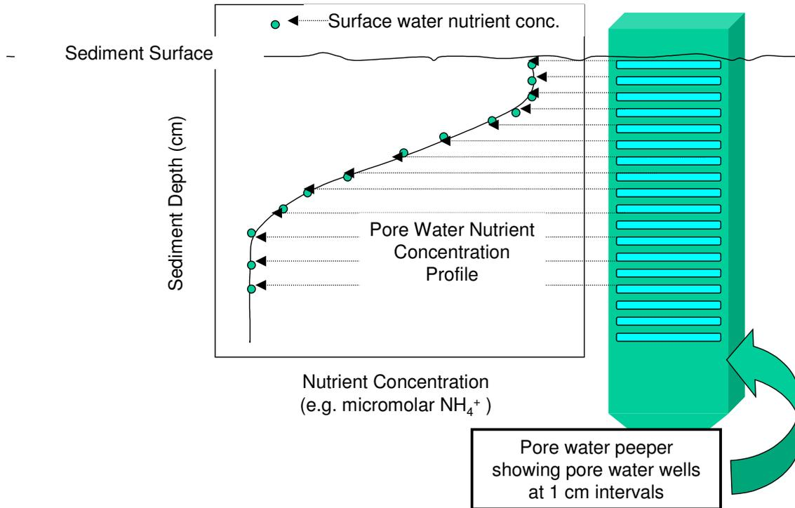
Figure 2-1. Graphic depicting how pore water profiles are generated from pore water peepers.
