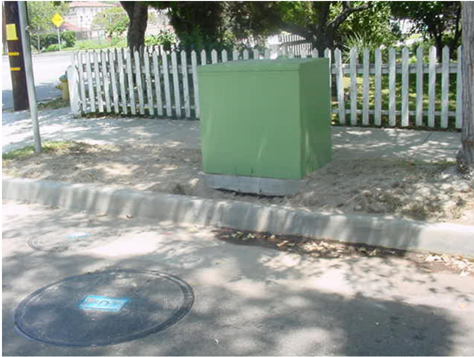
Figure 8. A. Autosampler contained within green housing box at the South Pasadena site. B. Housing containing the autosampler located next to the manhole cover of the CDS unit.
