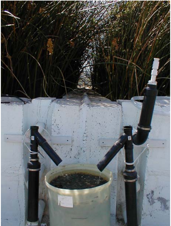
Figure 4. A. Dosing setup for the sub-surface flow wetlands at OCWD. Diazinon, Cu and Zn were added to the wetlands by peristaltic pumps. The metals stock solution is separate from the diazinon stock solution. B. Outflow from the two replicate cells.
