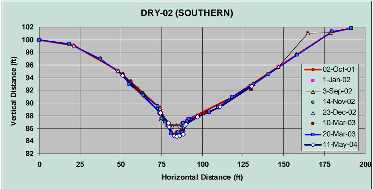
Fig. C3-15. Cross-Section of Dry Creek (2001 through 2004)
