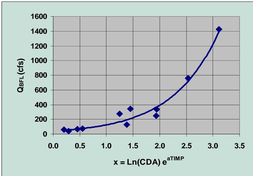
**Figure C4-8. Illustration of Fit to Dominant Discharge Values**
