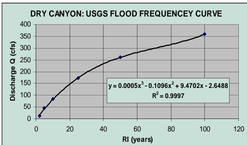
Fig. C2-12. Flood Frequency Curve For Dry Creek Using USGS Relations For the South Coastal Region of California
