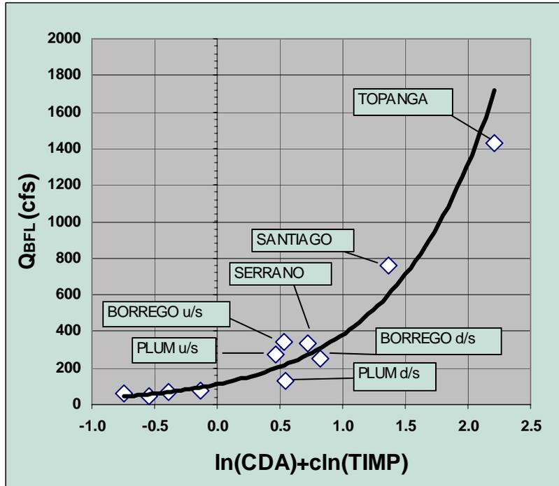
**Figure C4-7. Illustration of Fit to Dominant Discharge Values**
