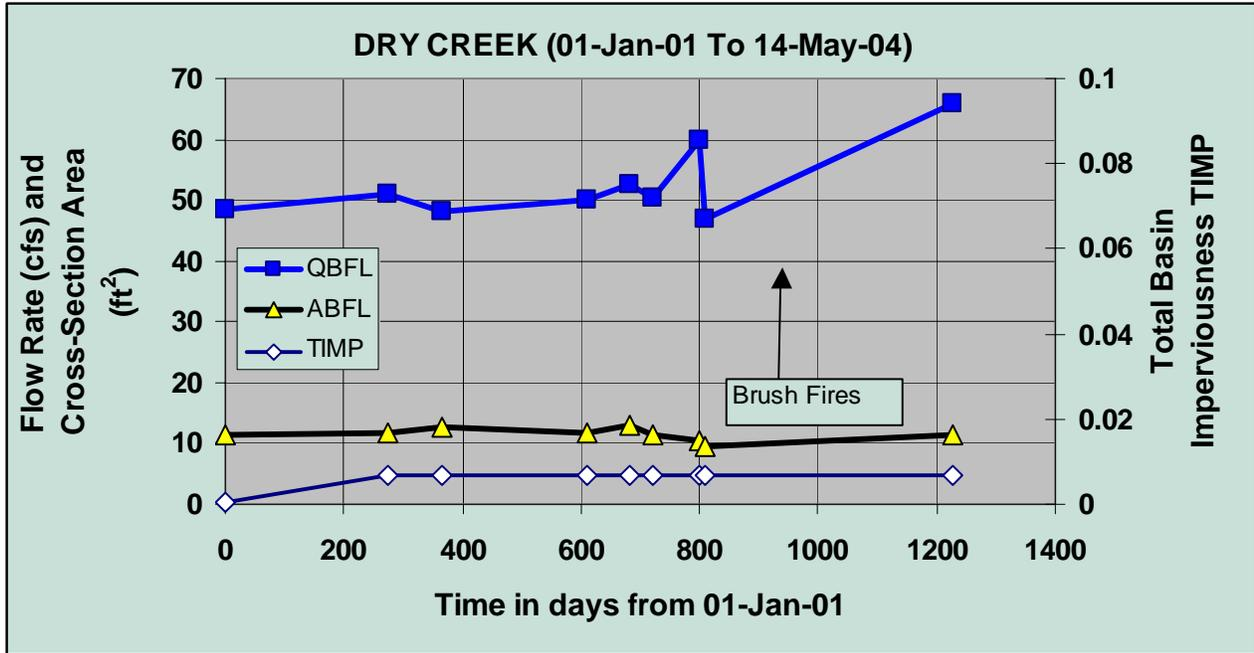
**Figure C4-3. Change in  $Q_{bfl}$ , Cross-Section Area and TIMP**
