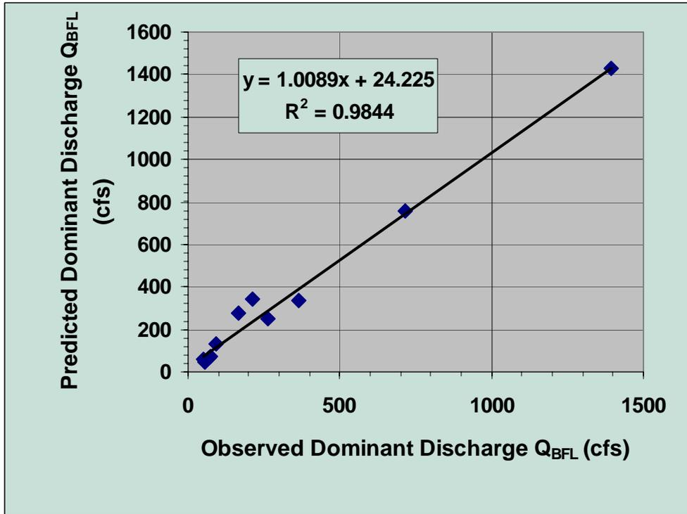
**Figure C4-9. Comparison of Predicted Flows to Observed Flows**
