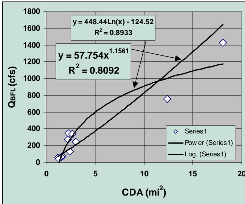
**Figure C4-5. Possible Models Based on Catchment Drainage Area**
