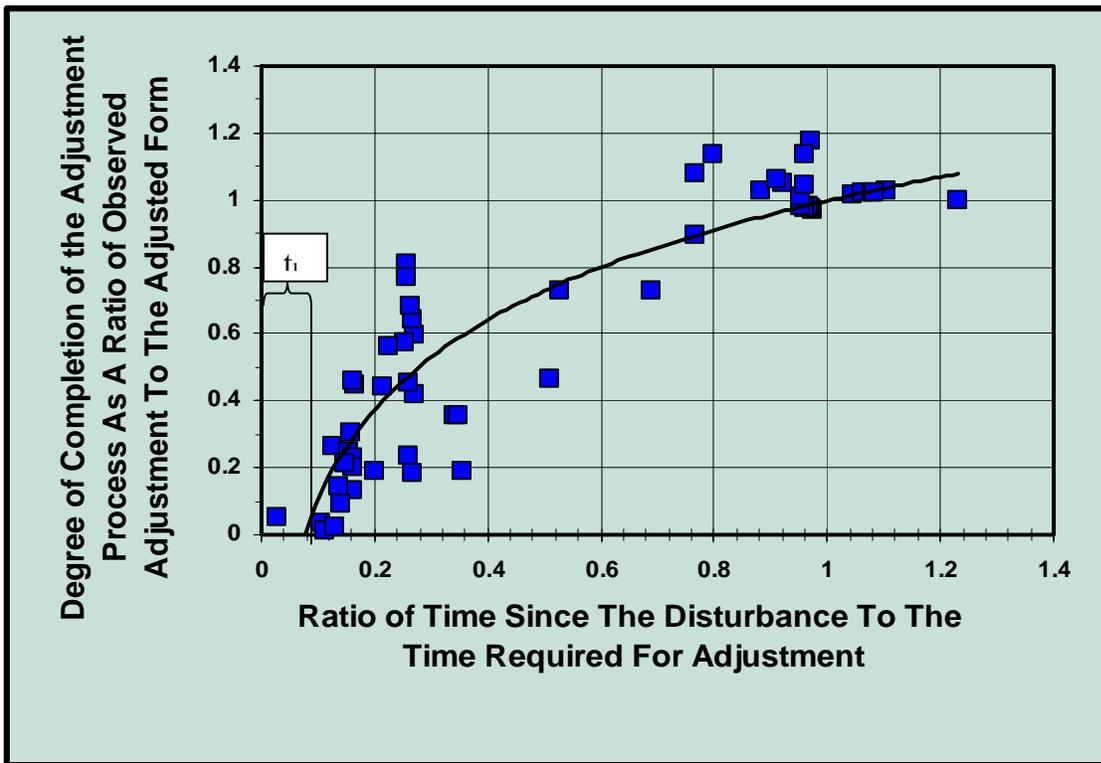
**Figure C4-4. Relaxation Curve for AL-Type Channels**
