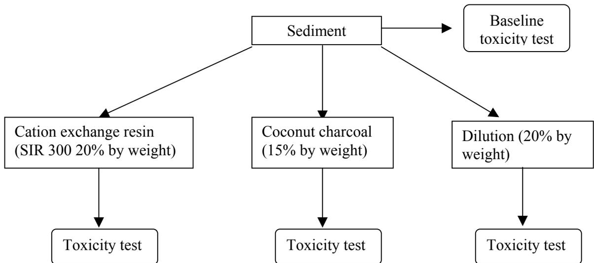
Figure 15. Schematic of sediment water interface, pore water and sediment TIE treatments.
