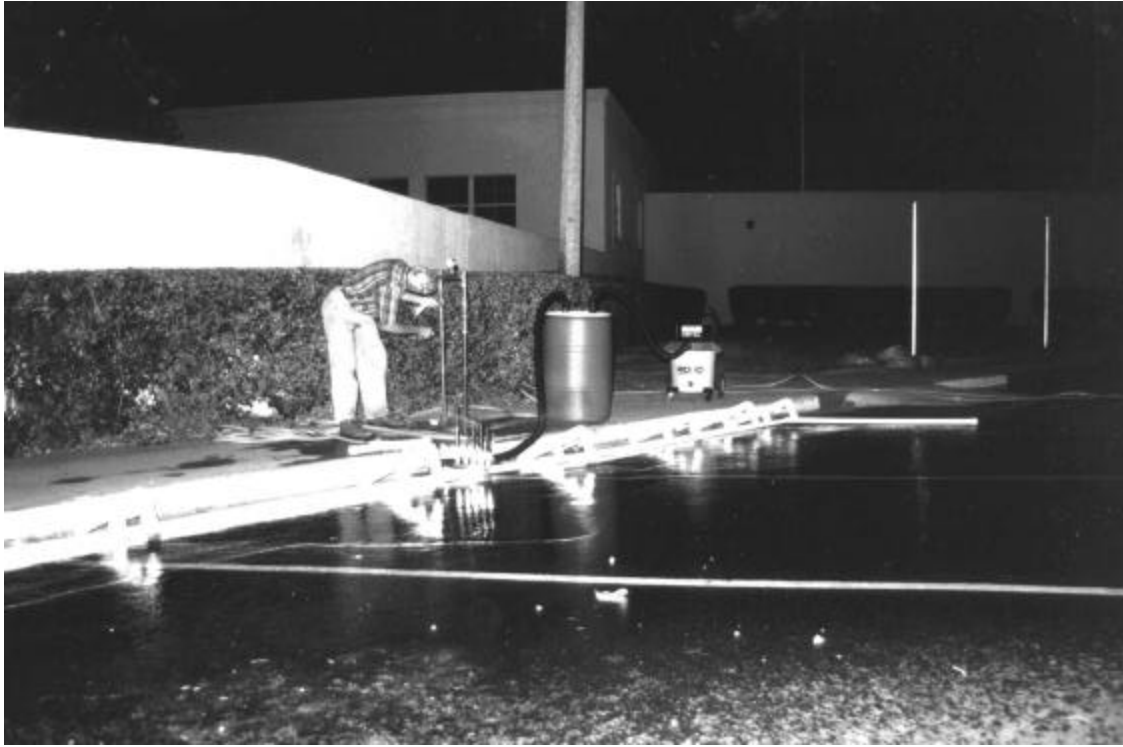
FIGURE II-2. The simulated rainfall delivery and water collection system used for assessing the effects of rainfall on surface runoff.
