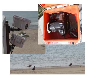
**Figure 4.** A computer controlled, high-frequency DSLR camera system deployed at Doheny State Beach collected images every three minutes to assess bird activity and density on the beach via change detection algorithms developed in MATLAB.
