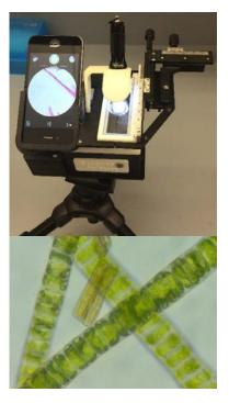
**Figure 3.** The SCCWRP CellScope, developed in collaboration with UC Berkeley, and a sample specimen image captured with an iPhone.
