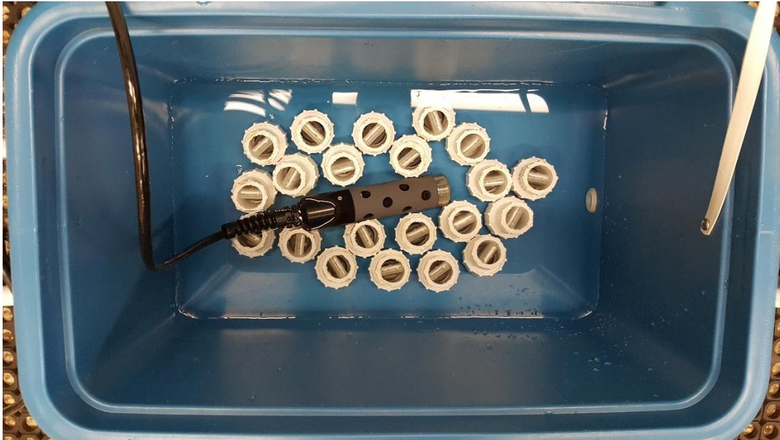
Image 3. The calibration test with a YSI meter and HOBO pendants properly submerged in conductivity solution within a container.
