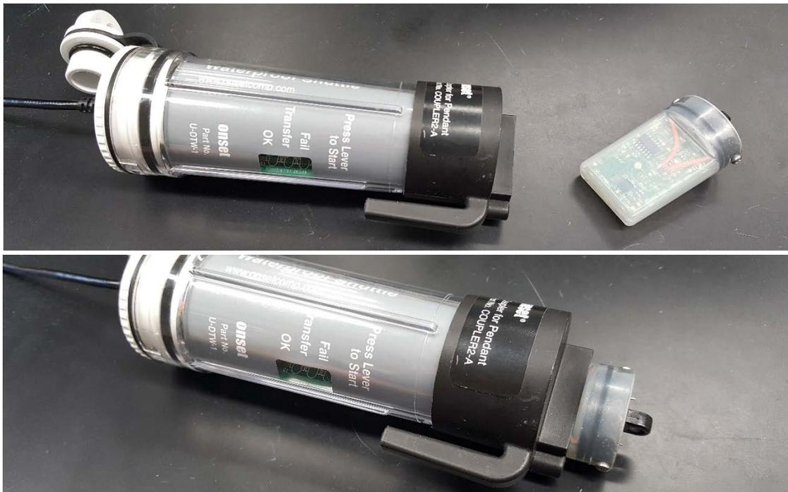
Image 1. HOBO pendant detached and attached to the waterproof launch shuttle
