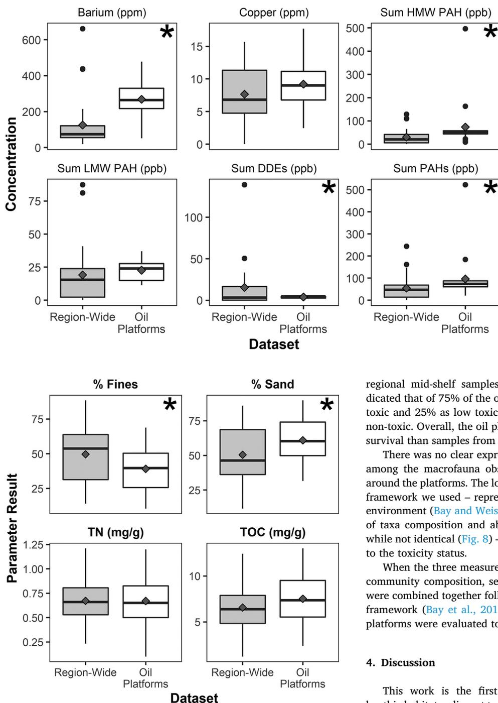
**Fig. 5.** Schematic box plots comparing measures of sediment grainsize composition (% Fines = %Mud + % Clay), total organic carbon (TOC), total nitrogen (TN) between oil platform samples and those from mid shelf depths across the Southern California Bight collected in 2013. An asterisk indicates a significant difference ( $\alpha = 0.1$ ) in a 1-way ANOVA test between the Regional and Oil Platform datasets. The grey diamonds indicate the mean value for each sediment parameter.
