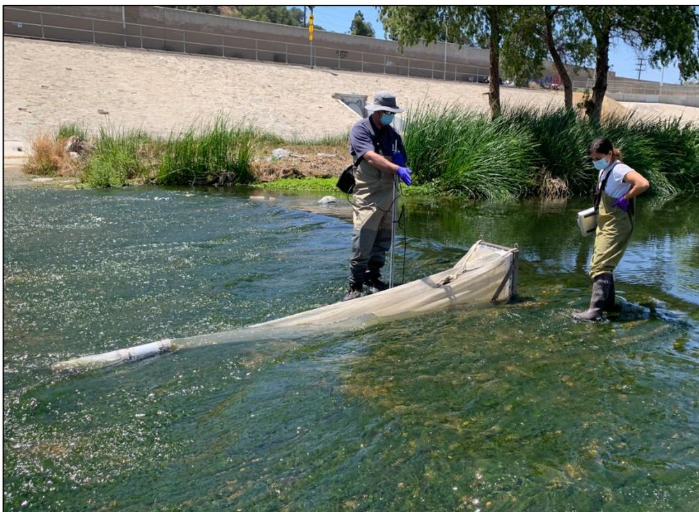
A SCCWRP field crew deploys a mesh sampling device known as a box frame net to collect microplastics from the Los Angeles River. As water flow through the net, microplastics and other particles become trapped at the far end. Researchers have begun working to standardize how microplastics are collected from aquatic environments.
