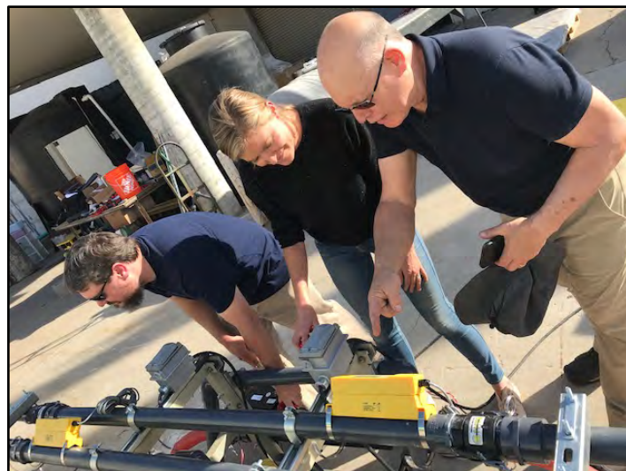
Clockwise from top right, SCCWRP researchers test a newly constructed sewer exfiltration test system on SCCWRP's patio; Dr. Joshua Steele, Dr. Amy Zimmer-Faust and Dr. John Griffith inspect yellow-colored, ultrasonic flow meters placed upstream and downstream of a sewer pipe that measure flows through the system; and Dr. John Griffith inspects the downstream end of a sewer pipe as clean water pours from it.
