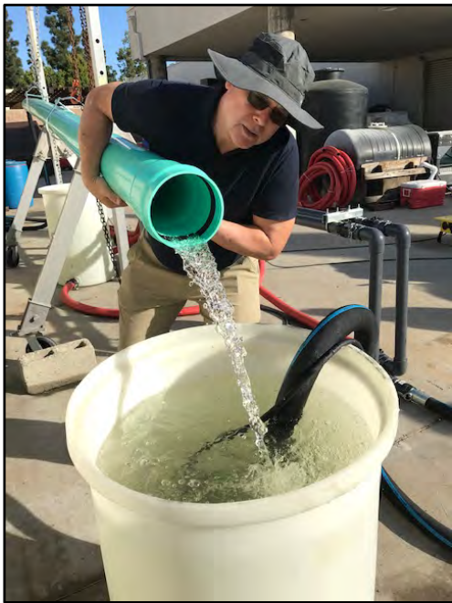
Clockwise from top right, SCCWRP researchers test a newly constructed sewer exfiltration test system on SCCWRP's patio; Dr. Joshua Steele, Dr. Amy Zimmer-Faust and Dr. John Griffith inspect yellow-colored, ultrasonic flow meters placed upstream and downstream of a sewer pipe that measure flows through the system; and Dr. John Griffith inspects the downstream end of a sewer pipe as clean water pours from it.
