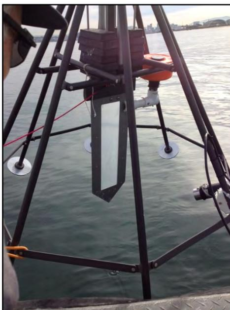
**A field crew deploys a passive sampling device into San Diego Bay for a study probing the origins of contamination found in fish in the bay. The device consists of a pointed metal frame containing polyethylene film that is inserted into the surface layer of sediment for a month. The device measure contaminant concentrations in the water between sediment particles, known as sediment pore water, and at the sediment-water interface just above.**
