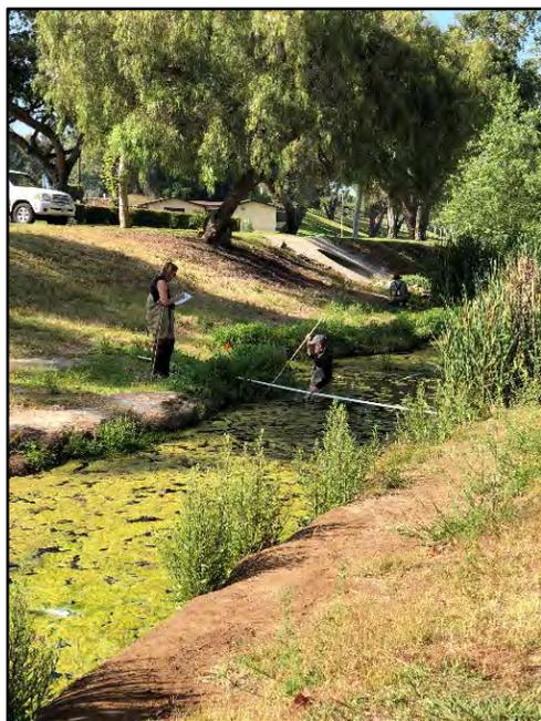
**A field crew from the Southern California Stormwater Monitoring Coalition (SMC) conducts a trash survey of Fullerton Creek in Orange County in June. The SMC is conducting trash surveys in streams across Southern California to support a Bight '18 study tracking the spread of trash in aquatic systems.**
