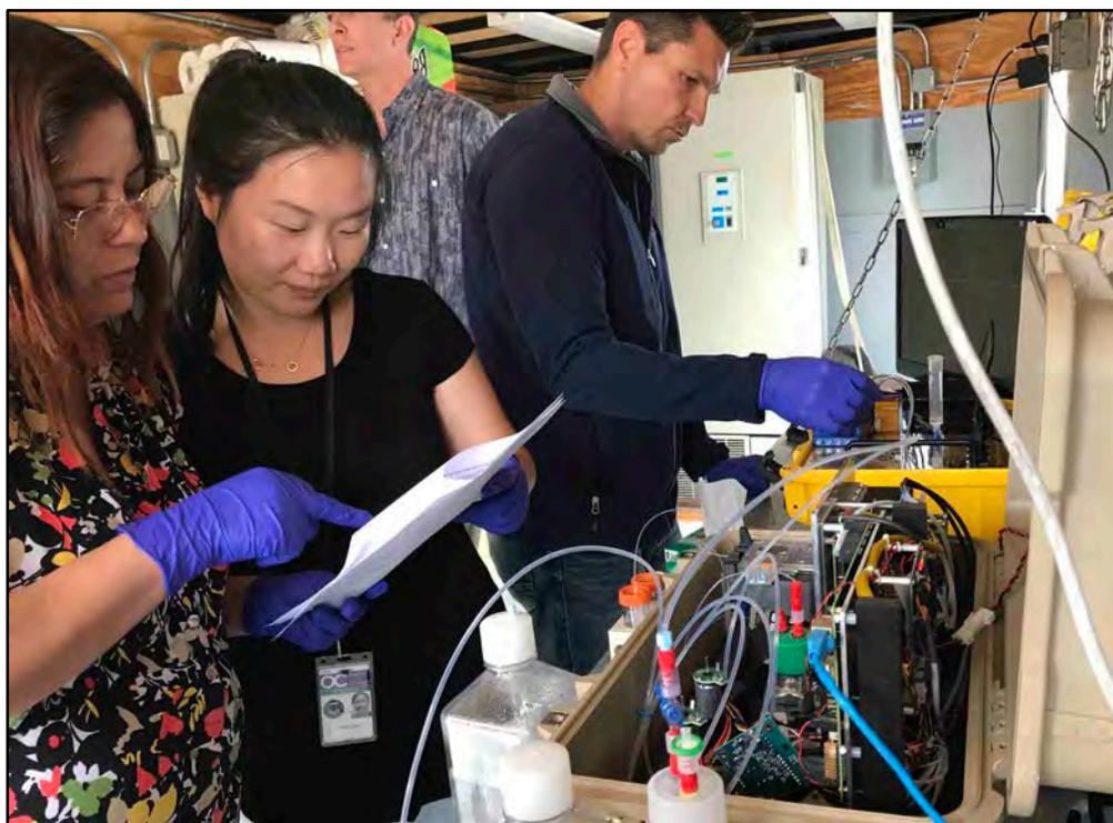
SCCWRP member agencies and other partners conduct field testing in May on a field-portable microbial detection device intended to improve the speed at which beach water can be analyzed. The field testers found that the instrument did not perform reliably; it will undergo further development. Pictured are Zaira Valdez of the City of San Diego, left, Stella Shao of Orange County Public Works, and Ryan Reinke of the Sanitation Districts of Los Angeles County.
