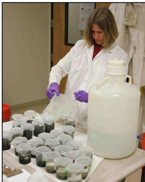
SCCWRP's Liesl Tiefenthaler prepares sediment samples collected from a site in Los Angeles Harbor for a toxicity identification evaluation (TIE) study. SCCWRP is working to optimize the design of sediment TIE studies to improve confidence in the results.
