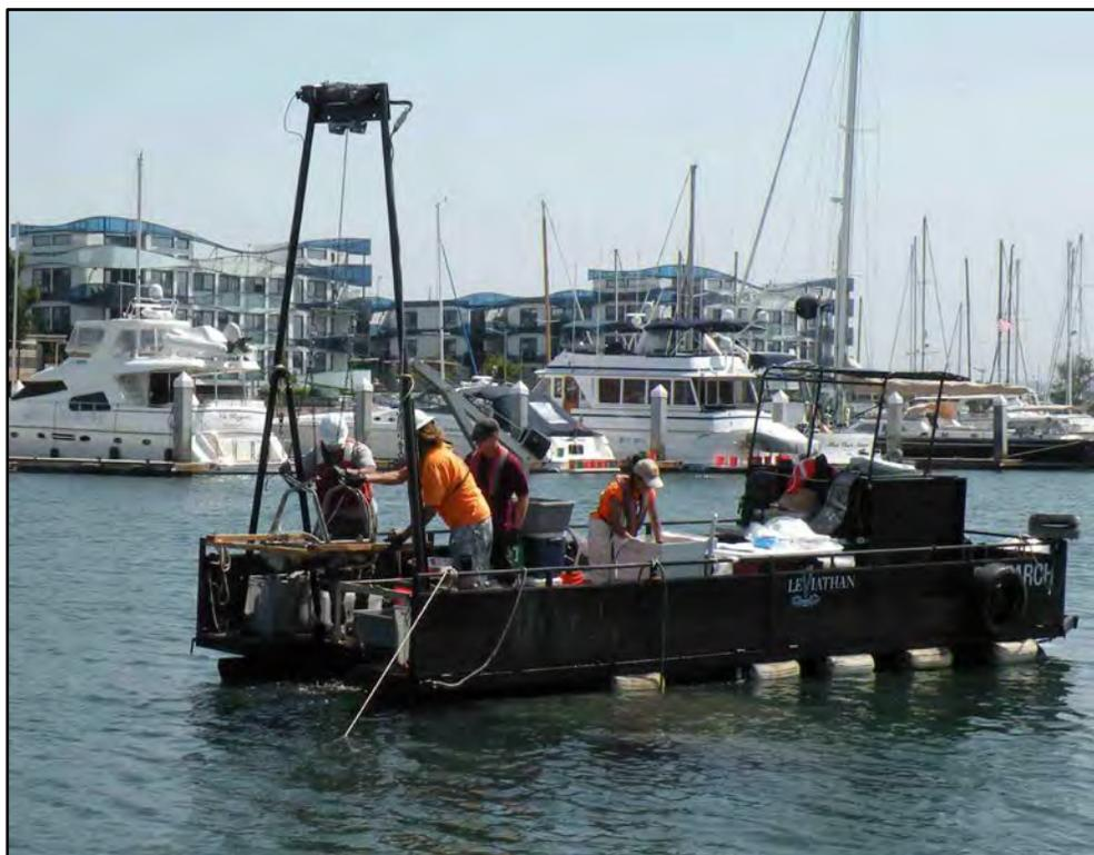
A field crew retrieves sediment grab samples from the bottom of Marina del Rey Harbor. The stressor identification study in the harbor has underscored the need for next-generation sediment Toxicity Identification and Evaluation (TIE) analysis methods.
