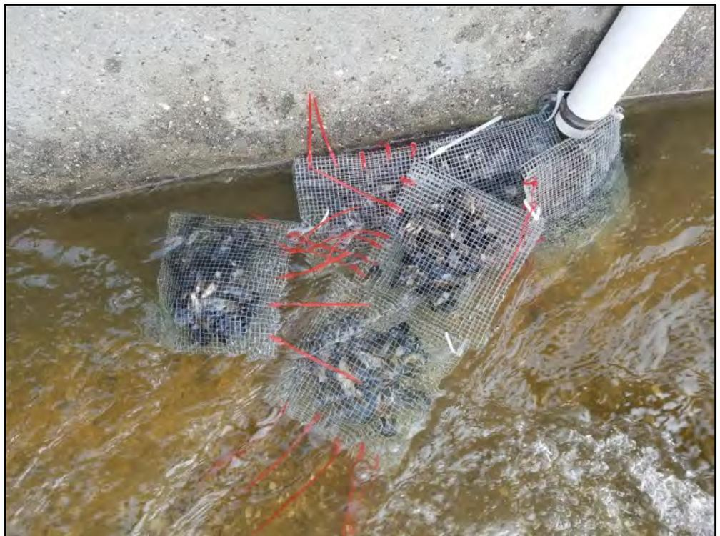
Mussels are placed in metal mesh bags and tied to a post in Coyote Creek in Orange County for a pilot study examining how long the organism's environmental DNA signal lingers following the removal of the organism.
