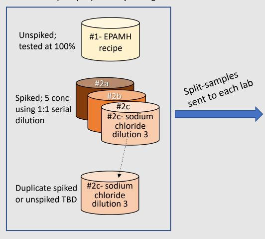
Experimental set up for each testing batch per lab
