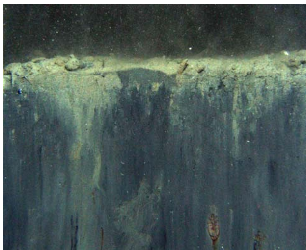
Figure 1. Sediment profile camera (left) and sediment profile image (right). Schematic of camera shows prism/carriage assembly that moves up or down relative to the frame so as to penetrate into the sediment and capture a picture. Image at right is 15 cm wide, taken in a Mid-Atlantic estuary. Infauna, animal tubes, and lighter oxidized sediments are visible.
