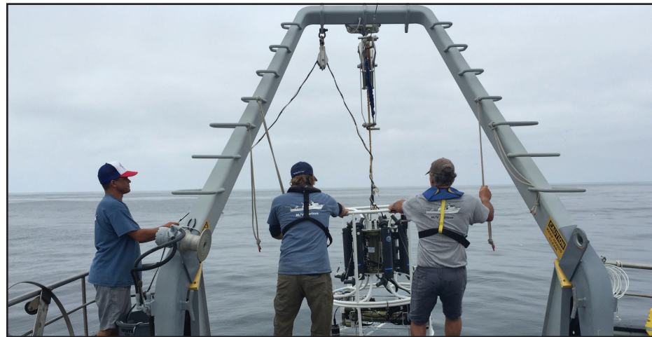
A field crew lowers a CTD (conductivity, temperature, depth) rosette into the ocean to take multiple measurements of seawater chemistry. The Southern California Bight Regional Monitoring Program has collected the first comprehensive ocean acidification data sets for Southern California's continental shelf.
