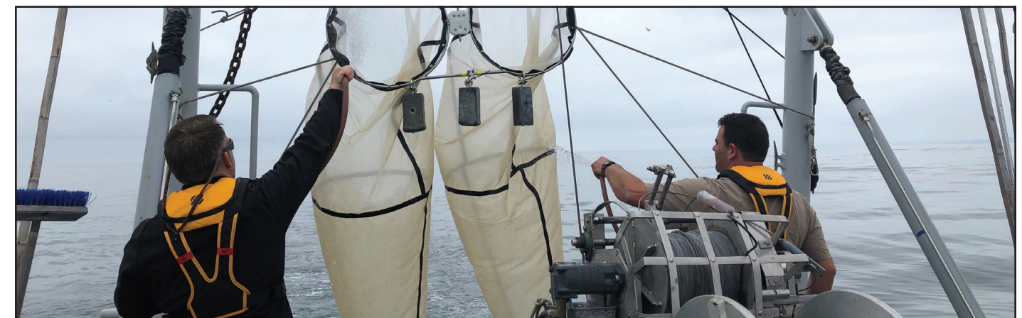
A pair of plankton nets is lowered into Southern California's coastal ocean to collect small, shell-forming marine organisms vulnerable to ocean acidification. The biological data explain how marine life already are being affected by seasonally corrosive coastal conditions.
