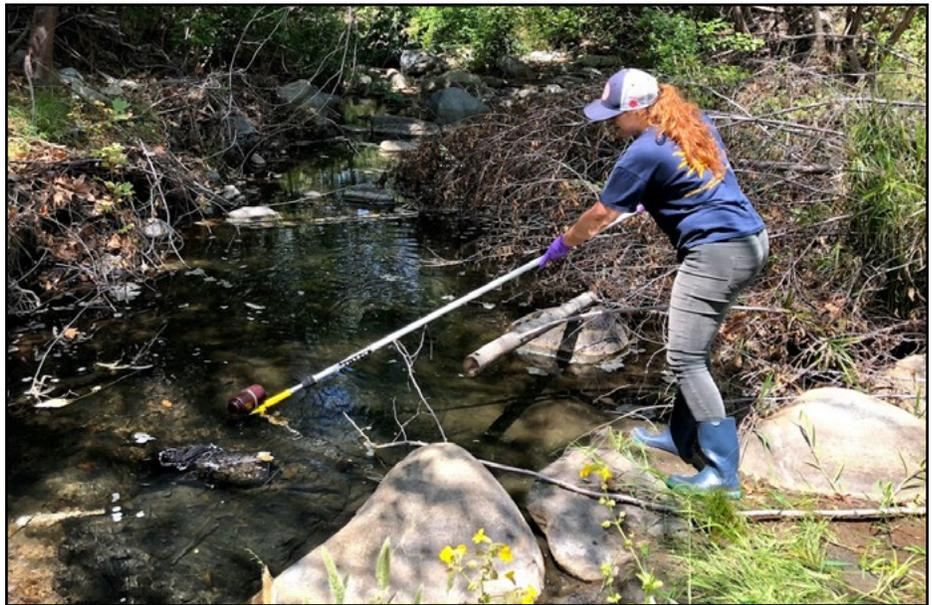
SCCWRP’s Dana Shultz collects a water sample in Upper San Juan Creek in San Diego County just a few feet from where mussels in metal cages have been temporarily placed into the stream. Researchers are investigating the feasibility of identifying organisms by the DNA they shed into their environment, known as environmental DNA.
