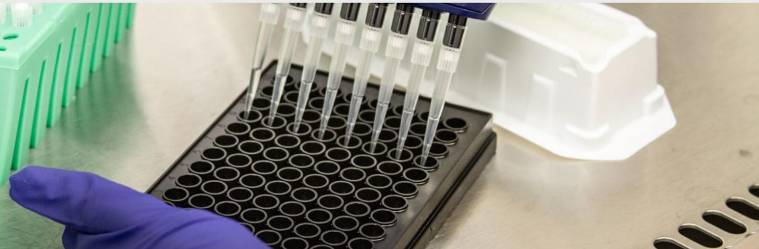
Laboratory-grown cells are placed into assay wells for bioanalytical screening, an approach that has the potential to help environmental managers monitor hundreds and perhaps thousands of chemical contaminants in aquatic systems.
