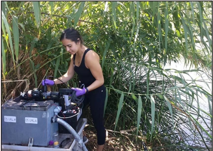
SCCWRP’s Syd Kotar monitors water quality inside a mobile unit that houses fish. The units, set up along the banks of the Los Angeles River, were used to expose the fish to flowing river water in real time, enabling researchers to track potential biological impacts from exposure.
