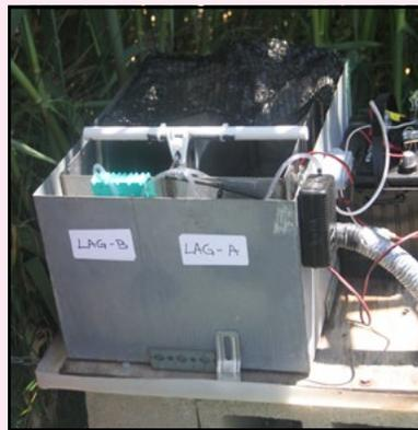
Fish that have been placed in mobile exposure units, above, are exposed to flowing Los Angeles River water in real time. Researchers are tracking whether fish are impacted by CECs in the water.
