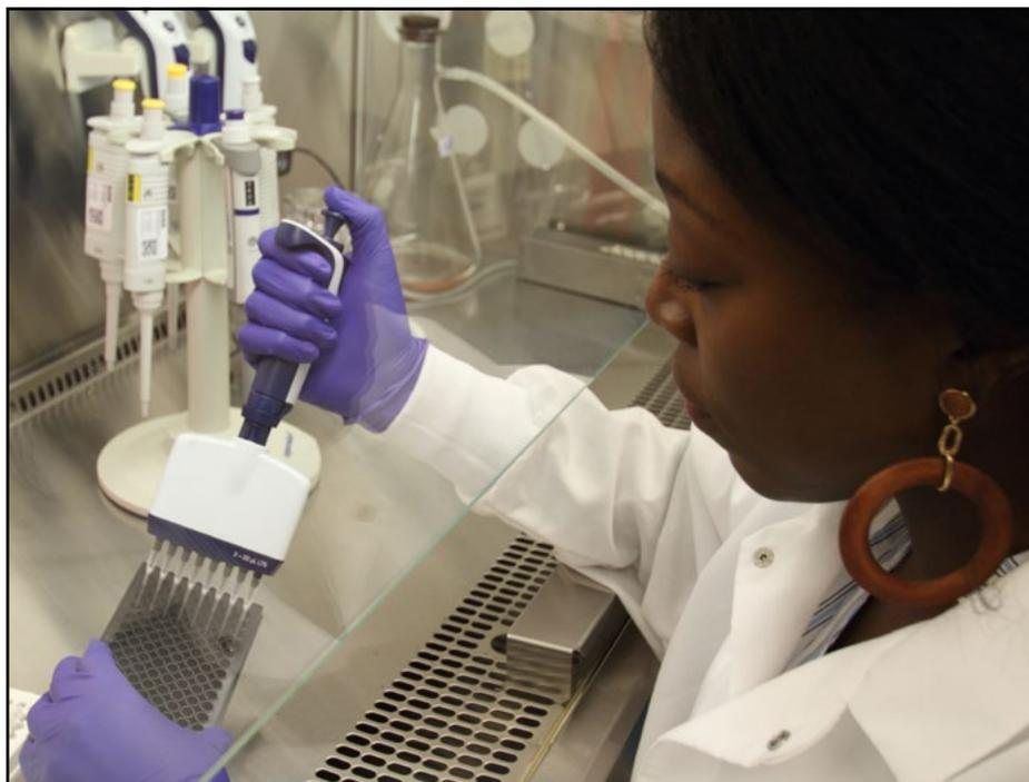
SCCWRP's Dr. Alvina Mehinto transfers small aliquots of cells into assay wells for a bioanalytical screening test that involves exposing the cells to a water extract sample, then tracking how they respond. Bioanalytical screening has the potential to enable water bodies to be screened for hundreds and perhaps thousands of chemical contaminants.
