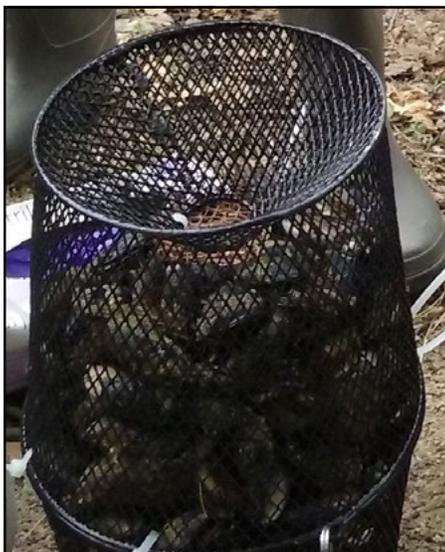
Mussels are placed into a metal cage in preparation for a study seeking to better understand how far and for how long the DNA they shed into their environment can be detected in the system.
