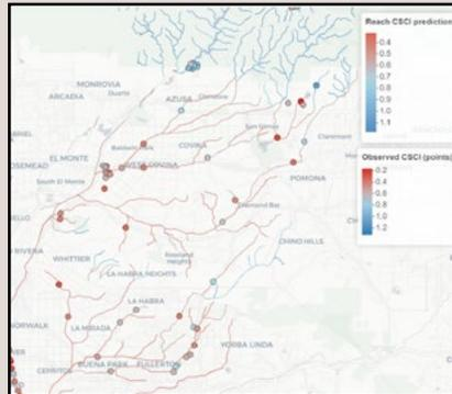
The Stream Classification and Priority Explorer (SCAPE) is a web app that helps stream managers visualize how stream biointegrity scores in a watershed are likely to be limited, or “constrained,” by urban and agricultural development. SCCWRP and its partners developed the app initially for use in the San Gabriel River watershed.
