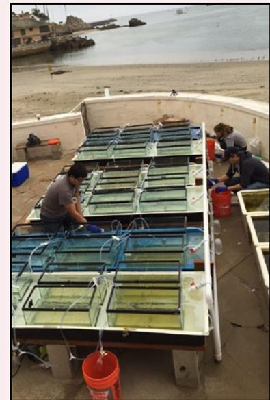
A mesocosm experiment is set up near the beach to examine the relative rates at which pathogens, fecal indicator bacteria and other microbes degrade in the environment. SCCWRP and its partners have shown that site-specific environmental factors can influence the rate at which different fecal microbes degrade.
