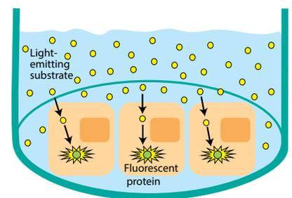
The strength of the signal reflects the CEC levels in the water sample.
