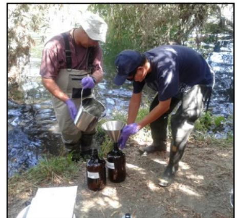
A SCCWRP field crew collects water samples to screen water bodies for chemical contaminants using multiple laboratory methods, including bioanalytical screening.
