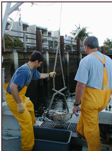
SCCWRP researchers use a grab sampler to collect surface sediment from the bottom of Newport Bay in Newport Beach.
