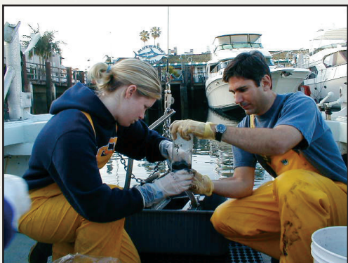
SCCWRP researchers collect sediment core samples from the silted bottom of Newport Bay in Newport Beach.
