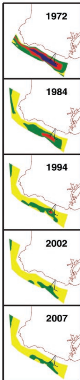
Figure 5. Organic nitrogen (% dry weight) in surface sediments (0 - 2 cm) off Palos Verdes 1972 to 2007. Selected years represent primary treatment (1972), advanced primary treatment (1984), partially secondary treatment (1994), full secondary treatment (2002), and most recent data (2007).
