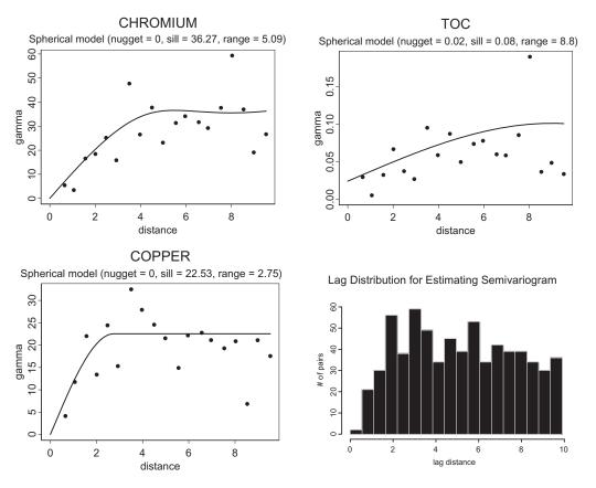
Figure 3. Empirical semivariograms and fitted models for three chemical constituents from PLWTP existing monitoring grid and the distribution of lags from PLWTP fixed monitoring grid. Fitted model and estimated parameters provided in subtitle. Distances are in kilometers.
