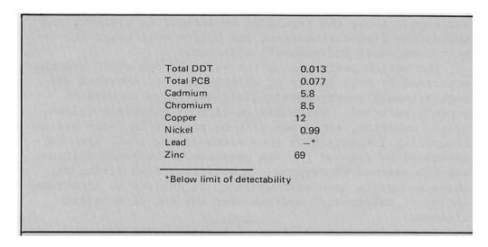
Table 2. Characteristics (mg/dry kg) of two samples of Palos Verdes sediments used in laboratory exposure tests.
